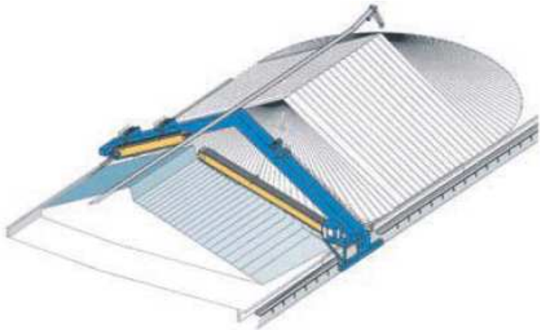
Longitudinal stockyard with twin-boom portal reclaimer
